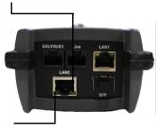
The green Speed LED and yellow Link/ Data LED indicate transmission speed
