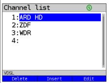
ARGUS initially displays the TV channels already selected in the set order that was tested for the IPTV scan. If no channels have been selected yet, the list is empty. The list slots can be filled one after another. You can select up to 250 channels.
